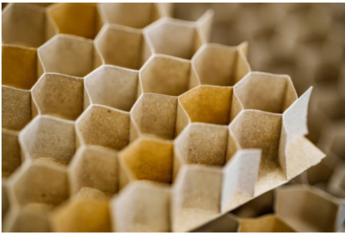
Close-up of the Honeycomb Structure. Cell size, paper quality and core height have a significant influence on the mechanical properties of the material.
