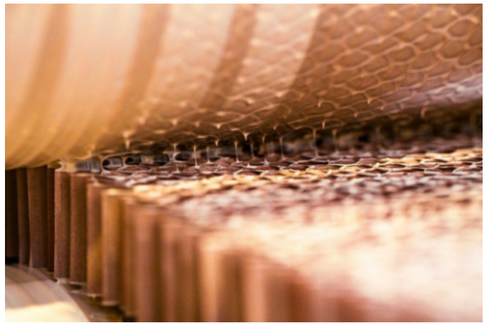
Application of Adhesive to the Expanded Honeycomb Core in Preparation for Subsequent Lamination with Paper Facing Sheets
